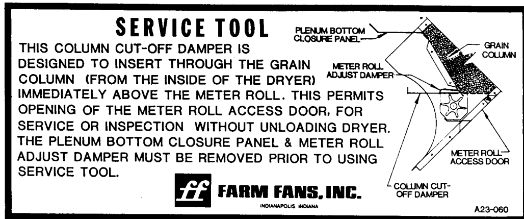
Fig. 6-16 Grain column cutoff damper decal showing installation
